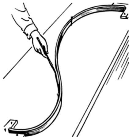
A spline, or the more modern term flexible curve, consists of a long strip fixed in position at a number of points that relaxes to form and hold a smooth curve passing through those points for the purpose of transferring that curve to another material. (Wikipedia)
