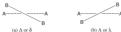
Figure IR-9.2. The figure shows pairs of non-orthogonal skew-lines in projection upon a plane parallel to both lines. The full line BB is above the plane of the paper, the dotted line AA is below this plane. Case (a) corresponds to (a) of Figure IR-9.1 and defines a right-handed helix. Case (b) corresponds to (b) of Figure IR-9.1 and defines a left-handed helix.
