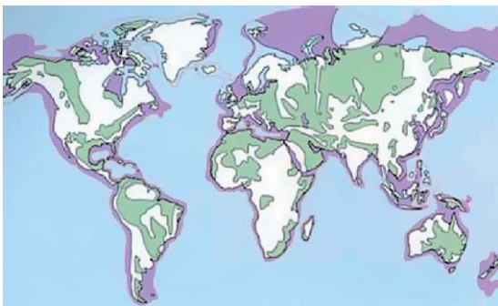
Figure 1 Sedimentary basins of the World. Onshore basins are shown in green, offshore basins are lavender and shown for a maximum water depth of 1000 m. Modified from Schlumberger (1991). World oil reserves – charting the future. Middle East Well Evaluation Review 10: 7–15.
