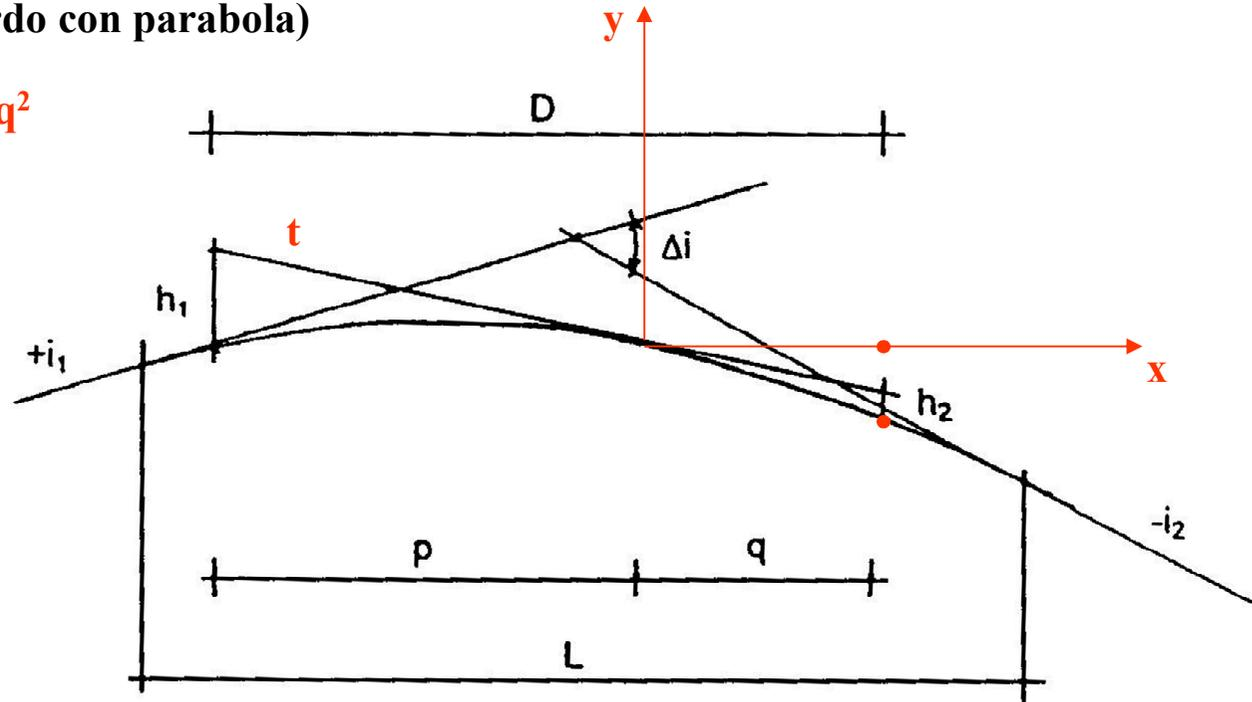
$$L = \frac{D^2 \cdot \Delta i / 100}{2 \cdot (h_1 + h_2 + 2 \times \sqrt{h_1 \times h_2})}$$
