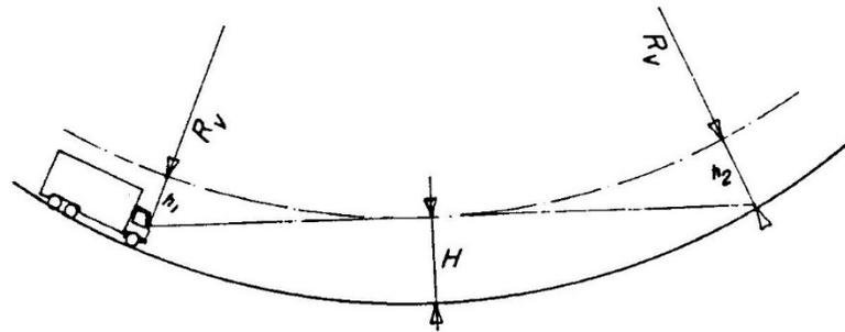
$$R_v = \frac{D^2}{2 \cdot (h_1 + h_2 + 2 \times \sqrt{h_1 \times h_2})}$$
