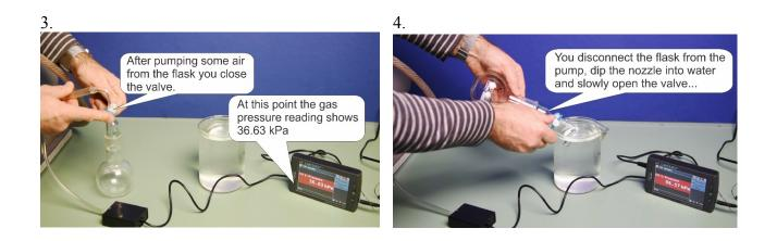
**a.** You determined that the total volume of the flask with the part before the valve is  $320 \pm 3$  ml. In the manual of the gas pressure sensor, you found that the instrumental uncertainty of the gas reading is  $\pm 3$  kPa.
