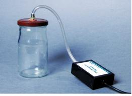
immerse the glass jar in water baths of temperatures  $T_2 = 1^{\circ}$ C and  $T_3 = 98^{\circ}$ C and record the corresponding gas pressure once it reaches a stable value:
