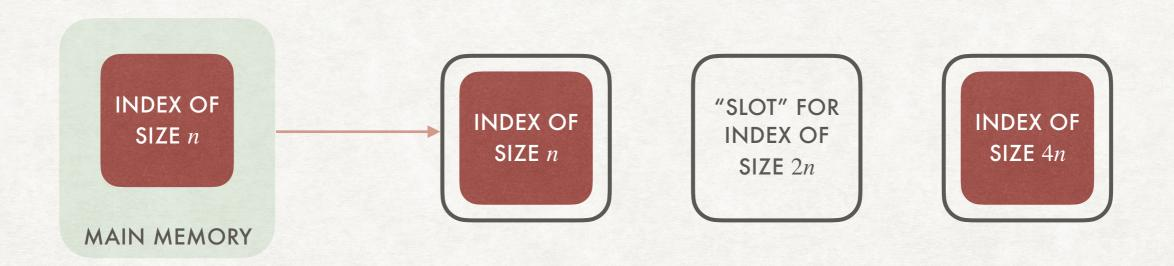
When full it is copied to disk. No merge is necessary (the "slot" is free) A new (empty) index of size n is created in memory
