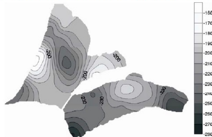
Figure 5 Map of the Eh sediment values in the Orbetello lagoon (data expressed in mV)
