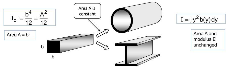
Define shape factor for elastic bending, measuring efficiency, as
