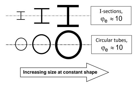
Each of these is roughly 10 times stiffer in bending than a solid square section of the same cross-sectional area
