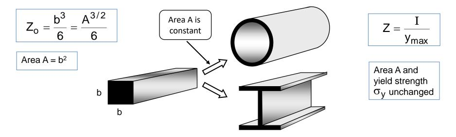
Define shape factor for onset of plasticity (failure), measuring efficiency, as
