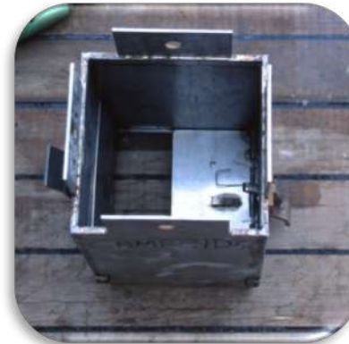
Core cutter and catcher
