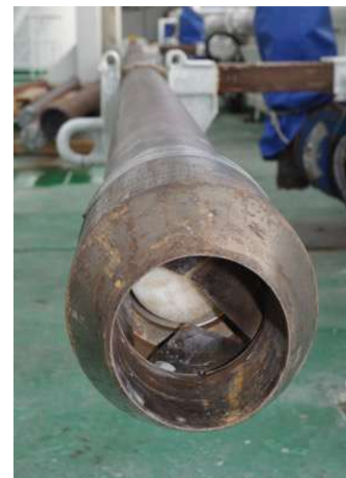
core cutter and catcher
