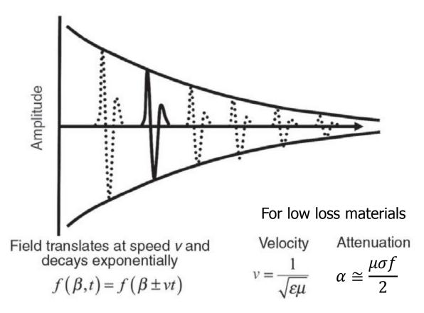
EM fields propagate as spatially damped waves when electrical losses are small. The signal amplitude decays exponentially in the direction of field translation while the field shape remains invariant.
