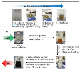
**Figure 35.** Photographs of steps involved in the preparation of CTAB-Au NRs, using wet chemical seed-mediated method (in the presence of sodium salicylate). (A) Preparation of CTAB-capped seeds. (B) Growth of CTAB-Au NRs.
