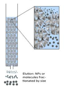
**Figure 56.** Principle of size exclusion chromatography. Small impurities enter the pores of gel beads and are thus retarded, whereas larger NPs are eluted faster.
