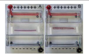
**Figure 61.** Recovering Au NPs from a gel band. (A) The extracted band contains Au NPs ( $\approx$ 4 nm diameter, cf. Section 1.2, Section 6.3) and was placed inside a dialysis bag, which was placed into the electrophoresis cell. (B) After applying an electric field the Au NPs migrated out of the gel band but remained trapped inside the dialysis bag.
