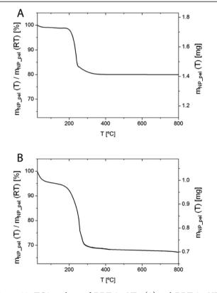
**Figure 80.** TGA analyses of DDT-Au NPs (A) and DDT-Au NPs overcoated with PMA (B). In both graphs,  $m_{\rm NP\_pel}(T)$  describes the mass of the NP pellet at temperature *T*. The masses are normalized to the mass  $m_{\rm NP\_pel}(\rm RT)$  at RT. The same scale in the left *y*-axis is used to facilitate the comparison. For both samples  $d_c = 4.3$  nm.
