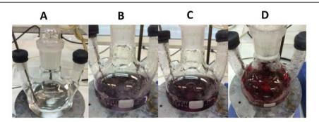
**Figure 32.** Synthesis of Cit-Au NPs of  $\approx$ 18 nm in diameter. Real photographs showing the color change at different stages: (A) before gold injection; (B) after injection of gold salt solution where the solution color changed to light blue and then to purple in (C), and finally to red color indicating the formation of Cit-Au NPs in (D).
