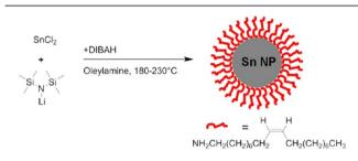
Figure 16. Synthesis of monodispersed Sn NPs.
