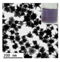
**Figure 73.** TEM image of hydrophilic star-shaped Au NPs (cf. Section 2.5) dried on a grid from a suspension of NPs in water. The scale bar corresponds to 200 nm. The inset shows glass vials filled with a suspension of star-shaped Au NPs.
