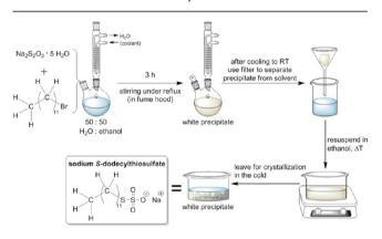
**Figure 11.** Schematic illustration of the chemical synthesis of sodium *S*-dodecylthiosulfate as a ligand precursor to stabilize Ag NPs.
