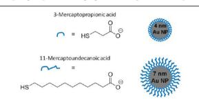
**Figure 45.** Sketch of the final Au NPs stabilized by MPA in case of  $d_c$  = 4 nm Au NPs and MUA in case of 7 nm Au NPs.
