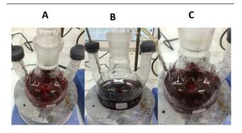
**Figure 33.** Synthesis of Cit-Au NPs of  $\approx 25$  nm in diameter using 18 nm seeds and the seed-mediated approach. Real photographs showing the color change at different stages: (A) 18 nm Au NPs seeds; (B) after injection of gold salt solution where the solution color changed to purple; and (C) after three injections (30 min reaction time between injections) to prepare Cit-Au NPs of 25 nm in diameter.
