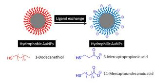
Figure 44. Ligand exchange on hydrophobic NPs (capped with hydrophobic ligands drawn in red) with hydrophilic ligands (drawn in blue). The chemical structures of 1-dodecanethiol, 3-mercaptopropionic acid, and 11-mercaptoundecanoic acid are shown.
