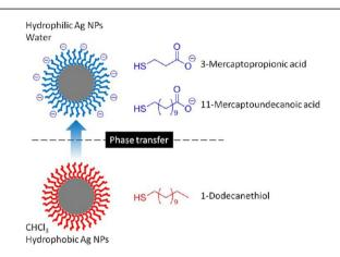
Figure 46. Phase transfer of DDT-Ag NPs from chloroform to water using 3-mercaptopropionic acid (MPA) or 11-mercaptoundecanoic acid (MUA).
