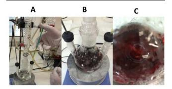
**Figure 29.** Synthesis of Cit-Au NPs of  $\approx 5$  nm in diameter. Photographs showing the reaction flask. (A) Before gold injection (note the yellow gold salt solution inside the syringe). (B) Immediately after injection of gold salt solution (the solution color changed from pale to purple in less than 10 s after the gold addition). (C) Few minutes (ca. 2 min) after injection of gold salt solution; the red color indicates the formation of the Cit-Au NPs.
