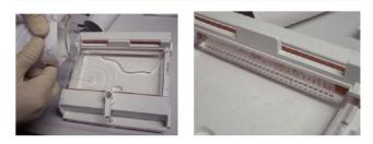
Figure 58. Boiling agarose solution is poured in the gel tray, and a template comb is inserted. The gel then is allowed to cool down and solidify at RT.
