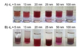
**Figure 41.** Phase transfer of PEG-Au NPs from water (upper layers in all vials) to chloroform containing DDT (lower layers in all vials). (A) Photographs of biphasic system after ligand exchange of Cit-Au NPs with PEG in water. (B) Photographs of biphasic system after phase transfer of PEG-Au NPs to the chloroform layer with DDT. Different vials correspond to Au NPs with different core diameters as labeled.
