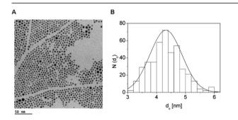
**Figure 64.** (A) TEM image of hydrophobic DDT-Au NPs (capped with dodecanethiol,  $\approx$ 4 nm core diameter, cf. Section 1.2) dried on a grid from a chloroform suspension. The scale bar corresponds to 50 nm. (B) Size distribution histogram, plotted as number of NPs  $N(d_c)$  that have a core diameter of  $d_c$ . From this histogram the mean NP diameter and its standard deviation was determined to be  $d_c = (4.3 \pm 0.4)$  nm.
