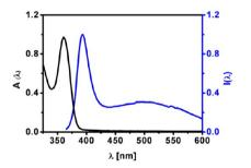
**Figure 98.** Normalized absorption spectrum  $A(\lambda)$  (black solid line, cf. Figure 94B) and emission spectrum  $I(\lambda)$  (blue solid line) of hydrophobic CdS NPs ( $d_c \approx 2$  nm, cf. Section 1.8) in toluene. The absorption and emission peaks, respectively, at  $\lambda_{abs} \approx 360$  nm and  $\lambda_{em} \approx 390$  nm correspond to CdS NPs of  $\approx 2$  nm.
