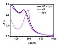
Figure 96. Normalized absorption spectra of  $\approx 4$  nm Au NPs (cf. Section 1.2: blue curve) recorded after their PMA coating and functionalization with a dye (cresyl violet perchlorate, CV) versus the spectrum free of the dye (red curve). The absorption at surface plasmon peak  $\lambda_{SPR} = 519$  nm of the NPs is normalized to  $A(\lambda_{SPR}) =$ 1.0. The absorption of the free dye at their emission maximum  $\lambda_{
