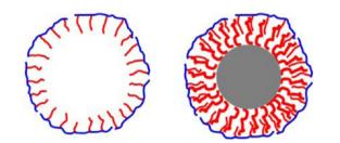
**Figure 51.** Empty polymer micelles (left) versus polymer-coated Au NPs (right). Due to similar size, separation using size exclusion chromatography is not efficient.
