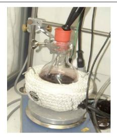
Figure 9. Au NPs are stirred after the addition of DDT while the temperature is controlled by a thermometer that is embedded in the reaction flask.
