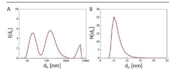
**Figure 104.** (A) DLS histograms of Au NPs of  $\approx 4$  nm coated with PMA measured in aqueous solution. (A) Intensity distribution  $I(d_h)$  and (B) number distribution  $N(d_h)$  of the hydrodynamic diameter  $d_h$ .
