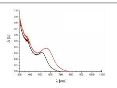
Figure 101. Absorption spectra of 5 nm core diameter Cit-Au NPs (purchased from BBI) as recorded in water (black curve) and in water supplemented with NaCl (red curve). The red shift of the SPR peak to higher wavelength and associated peak broadening is clear upon the addition of NaCl due to NP aggregation and plasmon coupling effect.
