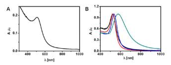
**Figure 90.** Normalized UV/vis absorption spectra of Cit-Au NPs (cf. Section 2.2) with core diameters of  $\approx$ 5 nm (A), 18 nm (B, black line), 25 nm (B, red line), 50 nm (B, blue line), and 100 nm (B, green line). The corresponding TEM images of these NPs are shown in Figure 70 A,D–G.
