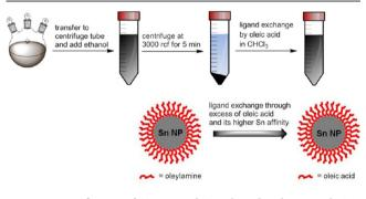
Figure 18. Purification of Sn NPs and OLA ligand exchange with OA.
