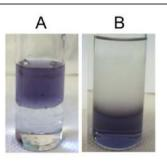
**Figure 43.** Phase transfer of star-shaped Au NPs from water (upper layers) to chloroform containing DDT (lower layers). Photographs of biphasic system before (A) and after (B) phase transfer from water to chloroform.
