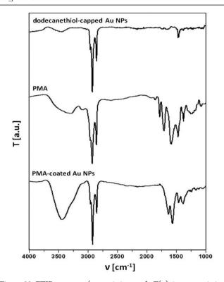
**Figure 82.** FTIR spectrum (transmission mode  $T(\nu)$ , i.e., transmission T versus wavenumber  $\nu$ ) of DDT-Au NPs of  $\approx$ 4 nm core diameter before and after overcoating with PMA. The spectrum of free PMA is shown as control.
