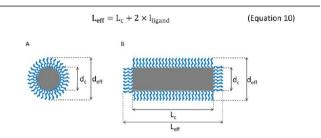
**Figure 28.** Sketch of (A) spherical and (B) rod-shaped inorganic NPs, comprising an inorganic core (drawn in gray) and an organic hydrophilic ligand shell (drawn in blue). In the case of nanorods, their shape is described by a cylinder with length  $L_c$  of the inorganic core and  $L_{\text{eff}}$  of the NP including the organic ligand shell and with diameter  $d_c$  of the inorganic core and  $d_{\text{eff}}$  of the whole NP.
