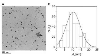
**Figure 67.** (A) TEM image of hydrophobic Sn NPs (capped with oleic acid,  $\approx 11$  nm core diameter, cf. Section 1.6) dried on a grid from a chloroform suspension. The scale bar corresponds to 200 nm. (B) Size distribution histogram, plotted as number of NPs  $N(d_c)$  that have a core diameter of  $d_c$ . From this histogram the mean NP diameter and its standard deviation were determined to be  $d_c = (10 \pm 4)$  nm.
