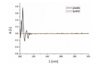
**Figure 86.** Absorption spectrum  $A(\lambda)$  of water (with water as blank) recorded in plastic or quartz cuvette. Note the cuvette-related absorption when a plastic cuvette was used at short wavelength.
