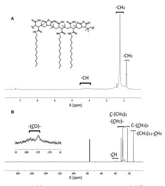
**Figure 83.** (A) <sup>1</sup>H NMR spectrum of PMA in  $CDCl_3$ . (B) <sup>13</sup>C NMR spectrum of PMA in  $CDCl_3$ ; the zoomed area shows the peaks for the carbonyl groups.
