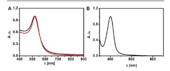
**Figure 89.** Normalized UV/vis absorption spectra of (A) Cit-Au NPs  $\approx$  13 nm core diameter (black line) versus Cit-Au NPs  $\approx$  20 nm core diameter (red line). (B) Cit-Ag NPs  $\approx$  15 nm core diameter. Au NPs and Ag NPs suspensions in water were prepared as detailed in Section 2.2 and Section 2.3, respectively.
