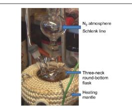
Figure 23. Reaction setup used for heating the mixture of CdO, oleic acid, and ODE.
