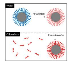
**Figure 40.** Hydrophobization of Au NPs via two-stage functionalization: (1) PEGylation in water (upper panel) by displacement of hydrophilic ligands (drawn in blue) by PEG-SH molecules (drawn in light red), followed by phase transfer into chloroform containing alkylamines (drawn in dark red).
