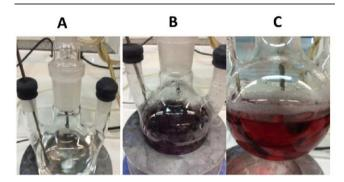
Figure 31. Synthesis of Cit-Au NPs of  $\approx 13$  nm in diameter. Photographs showing the reaction flask (A) before gold injection, (B) after injection of gold salt and EDTA solutions when the solution color changed to purple/blue, and (C) shortly (ca. 1 min) after injection, when the red color showed up, indicating the formation of Cit-Au NPs.
