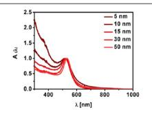
**Figure 91.** Normalized UV/vis absorption spectra of commercial Cit-Au NPs in water from BBI solutions (cf. Section 2.2) with core diameters of 5, 10, 15, 30, and 50.
