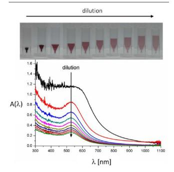
**Figure 87.** Concentrated aqueous solution of Au NPs was stepwise diluted, which can be seen by the fading color in the solution (upper panel) and deceasing absorption intensity (lower panel). High NP concentration (black curve) resulted in high absorption, and thus  $\lambda_{max}$  cannot even be identified due to detector saturation that results in peak broadening and distortion.
