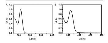
**Figure 94.** (A) Normalized UV/vis absorption spectrum of CdSe/ZnS quantum dots with core diameter of  $\approx 4$  nm (cf. Section 1.7; Figure 68) as recorded in toluene with  $\lambda_{max} = 516$  nm. (B) Normalized UV/ vis absorption spectrum of CdS quantum dots with core diameter of  $\approx 2$  nm (cf. Section 1.8; Figure 69) as recorded in toluene with  $\lambda_{max} = 360$  nm.
