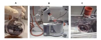
**Figure 50.** Phase transfer of DDT-Au NPs ( $d_c = 4.2$  nm) from chloroform to water using PMA-*g*-dodecyl polymer. Photographs of (A) DDT-Au NPs in chloroform after addition of the polymer solution dissolved in chloroform, (B) chloroform evaporated using a rotary evaporator, and (C) sonication after the addition of sodium borate buffer (pH 12).
