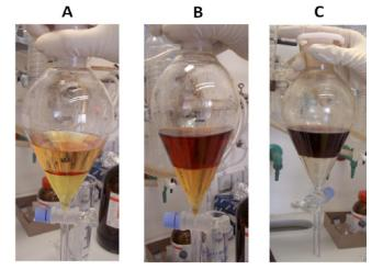
**Figure 3.** Photographs of the biphasic system showing the process of transferring  $AuCl_4^-$  ions from the aqueous phase (lower phase) to the organic phase (upper phase) through the formation of tetraoctylammonium tetrachloroaurate ion pairs (dark red phase in C).
