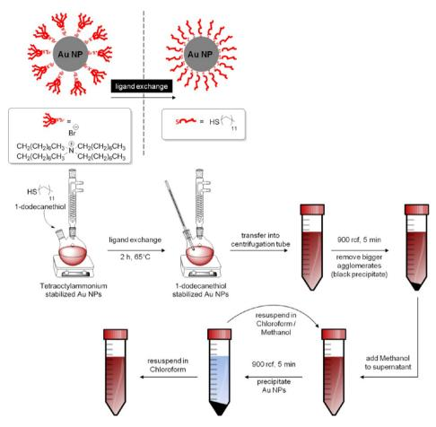
Figure 8. Ligand exchange on TOAB-Au NPs with dodecanethiol leading to the formation of DDT-stabilized Au NPs.
