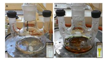
**Figure 34.** Synthesis of Cit-Ag NPs of  $\approx 15$  nm in core diameter. Photographs showing the solution color (A) before and (B) after injection of silver nitrate solution. Yellow solution color in B indicates the formation of Cit-Ag NPs. For more clarity, a photograph of a cuvette containing the solution is given in the inset.
