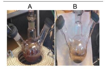
Figure 24. Color change of the mixture before (A) and after (B) decomposition of CdO.
