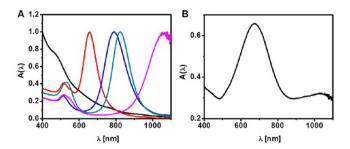
**Figure 92.** Normalized UV/vis absorption spectra of (A) Au NRs (cf. Section 2.4), with  $\lambda_{SPR} = 650$  nm (red curve), 790 nm (blue curve), 825 nm (green curve), 1050 nm (pink curve), and the original spherical Au seeds used to grow the nanorods (black curve). For TEM images of these Au NRs cf. Figure 72. (B) Star-shaped Au NPs with  $\lambda_{SPR} = 690$  nm (cf. Section 2.5). For TEM images of these NPs cf. Figure 73.
