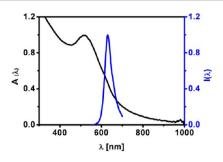
**Figure 99.** Normalized absorption spectrum  $A(\lambda)$  (black solid line, cf. Figure 96) and emission spectrum  $I(\lambda)$  (blue solid line) of hydrophilic Au NPs coated with PMA modified with cresyl violet (CV) ( $d_c \approx 4$  nm, cf. Section 1.2) as recorded in water. The absorption and emission peaks are at  $\lambda_{abs} \approx 519$  nm and  $\lambda_{em} \approx 630$  nm, respectively.
