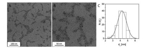
Figure 66. TEM image of hydrophobic Fe<sub>3</sub>O<sub>4</sub> NPs (capped with OA and OLA,  $\approx$ 4 nm core diameter, cf. Section 1.5) dried on a grid from a chloroform suspension. (A) The scale bar corresponds to 100 nm, and (B) the scale bar corresponds to 50 nm. (C) Size distribution histogram, plotted as number of NPs  $N(d_c)$  that have a core diameter of  $d_c$ . From this histogram the mean NP diameter and its standard deviation were determined to be  $d_c = (4.2 \pm 0.6)$  nm.
