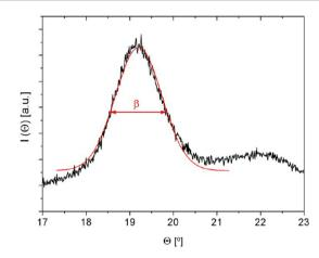
**Figure 79.** XRD diagram  $I(\Theta)$  of the (111) plane of polymer coated Au NPs ( $\approx$ 4 nm core size, cf. Section 1.2 and Section 6.3). The red line represents the GauSamp fit of the peak. This graph is a part of the graph shown in Figure 78.
