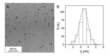
**Figure 65.** (A) TEM image of hydrophobic FePt NPs (capped with OA and OLA,  $\approx$ 4 nm core diameter, cf. Section 1.4) dried on a grid from a chloroform suspension. The scale bar corresponds to 100 nm. (B) Size distribution histogram, plotted as number of NPs  $N(d_c)$  that have a core diameter of  $d_c$ . From this histogram the mean NP diameter and its standard deviation were determined to be  $d_c = (3.4 \pm 0.6)$  nm.
