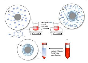
**Figure 39.** (A) Cit-Au NPs in solution with physically adsorbed and excess free citrate molecules. (B) Addition of mPEG-SH at basic pH to promote displacement of citrate molecules by mPEG-SH. (C) Purification by centrifugation in which PEGylated NPs are purified from free citrate molecules and mPEG-SH in the supernatant.
