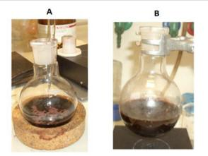
Figure 5. Reduction process of gold ions by sodium borohydride.
