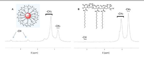
Figure 84. (A) <sup>1</sup>H NMR spectrum of PMA coated Au NPs of  $\approx$ 4 nm core diameter in 15% D<sub>2</sub>O/H<sub>2</sub>O mixture. (B) <sup>1</sup>H NMR of PMA in 15% D<sub>2</sub>O/H<sub>2</sub>O mixture after treatment with base to open all anhydride groups.
