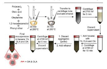
Figure 15. General scheme of the synthesis and purification of  $Fe_3O_4$  NPs. After the initial synthesis, both large aggregates and solvent impurities are removed by centrifugation, obtaining NPs that are finally stabilized by OLA and OA.
