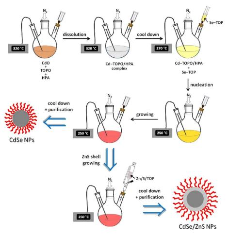
Figure 21. Schematic illustration of the synthesis of CdSe and CdSe/ZnS NPs.
