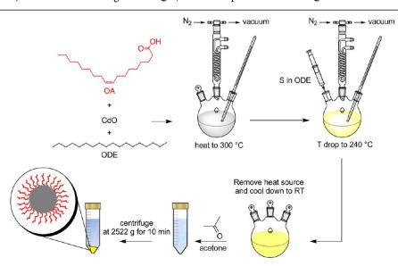
Figure 26. Schematic illustration of the chemical synthesis of hydrophobic CdS NPs ( $d_c \approx 2$  nm) is shown. OA, CdO, and ODE were mixed and heated at 300 °C resulting in a color change from brown to transparent. The sulfur solution in ODE was rapidly injected to induce the formation of NPs as evident from the change from transparent to light yellow (QDs). The QDs were purified (1–3 times) by addition of acetone or methanol followed by precipitation and centrifugation.
