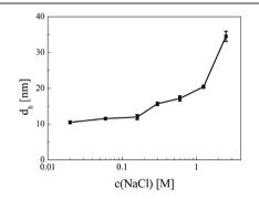
**Figure 105.** Hydrodynamic diameter  $(d_h)$  of 4 nm PMA-Au NPs as a function of NaCl concentration in the NP suspension.
