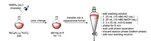
Figure 4. Synthesis of 4 nm TOAB-Au NPs is based on the reduction of Au(III) to elemental Au(0) by the addition of  $NaBH_4$ . After the formation of Au clusters, the NP suspension is washed several times with aqueous solutions.
