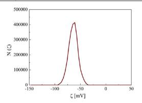
**Figure 108.** Distribution  $N(\zeta)$  of the zeta-potential  $\zeta$  as measured in water from a sample of  $\approx$ 4 nm core diameter PMA-Au NPs with  $c_{\rm NP}$ = 10 nM. The obtained mean value for the zeta potential is -48.07 ± 1.16 mV.
