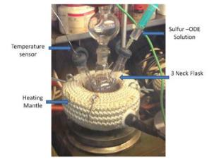
Figure 25. Injection of the sulfur-ODE solution at 300 °C.
