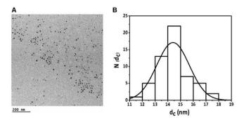
**Figure 71.** (A) TEM image of Cit-Ag NPs (cf. Section 2.3) dried on a grid from a suspension of NPs in water. The scale bar corresponds to 200 nm. (B) Size distribution histogram, plotted as number of NPs  $N(d_c)$  that have a core diameter of  $d_c$ . From this histogram the mean NP diameter  $d_c$  and its standard deviation were determined to be  $d_c = (15 \pm 1)$  nm.
