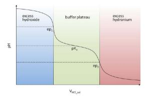
**Figure 110.** Illustrative titration curve of carboxylate stabilized NPs suspended in NaOH (aq) with the original volume  $V_{\text{NaOH}\_sol}$  against HCl (aq), of which the volume  $V_{\text{HCl}\_sol}$  has been added. The figure is adapted and modified with permission from Charron et al.<sup>61</sup> Copyright 2012 American Chemical Society.
