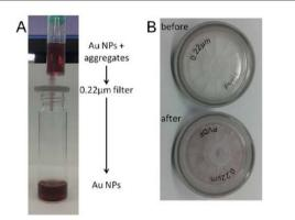
**Figure 52.** (A) Purification of PMA-g-dodecyl capped Au NPs ( $\approx$ 4 nm core diameter, cf. Section 1.2, Section 6.3) from aggregates via filtration using a syringe filter. (B) After filtration the aggregates can be seen in the filter by the naked eye.
