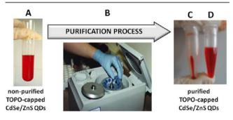
Figure 22. Purification process of the CdSe or CdSe/ZnS QDs by centrifugation and washing with methanol. (A) Vial with NPs dispersed in chloroform. (B) Centrifugation of the NP suspension after the addition of methanol. (C) Precipitated QDs after centrifugation. (D) QDs solution after removal of supernatant in C and redispersion in chloroform.
