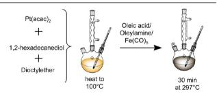
Figure 13. Schematic illustration of the chemical synthesis of 4 nm core diameter FePt NPs. The synthesis was carried out under water exclusion and  $N_2$  atmosphere in a three neck flask equipped with seal septa to be able to add all reagents under oxygen and water free conditions.
