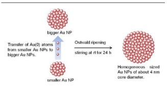
**Figure 7.** Ostwald ripening phenomena result in TOAB-Au NPs with a narrow size distribution. Smaller Au NPs in inhomogeneous population in terms of size dissolve and end up in bigger Au NPs.
