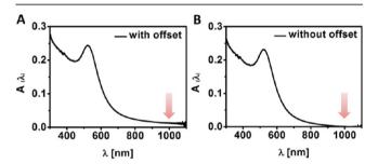
**Figure 85.** Absorption spectra (absorption (A) as a function of the wavelength  $\lambda$ ) of  $\approx$ 4 nm core diameter Au NPs (cf. Section 1.2) coated with PMA in water (cf. Section 6.3). (A) The "raw spectra" include an offset at higher wavelengths. (B) Processed spectra by subtracting the absorption at higher wavelengths from the whole spectra. Processed spectra provide more accurate comparison between different spectra with different offset levels.
