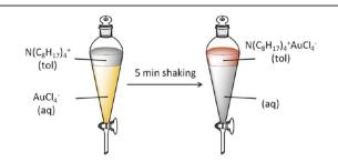
Figure 2. Scheme of the process of transferring  $AuCl_4^-$  ions from the aqueous phase to the organic phase through the formation of tetraoctylammonium tetrachloroaurate ion pairs.
