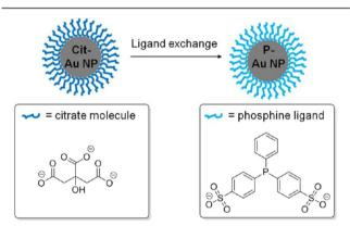
**Figure 38.** Scheme of the ligand exchange on Cit-Au NPs of different size with bis(*p*-sulfonatophenyl)-phenylphosphine. Spherical Cit-Au NPs of  $d_c = 5$  and 10 nm core size stabilized by citrate molecules (drawn as dark blue ligands) were modified by bis(*p*-sulfonatophenyl)-phenylphosphine molecules (drawn as light blue ligands). The resulting P-Au NPs have improved colloidal stability.
