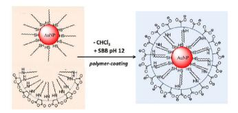
Figure 49. Phase transfer of DDT-Au NPs from chloroform (left) to water (right) using PMA-g-dodecyl polymer.
