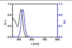
**Figure 97.** Normalized absorption spectrum  $A(\lambda)$  (black solid line, cf. Figure 94A) and emission spectrum  $I(\lambda)$  (blue solid line) of hydrophobic CdSe/ZnS NPs ( $d_c \approx 4$  nm, cf. Section 1.7) in toluene. The absorption and emission peaks are at  $\lambda_{abs} \approx 516$  nm and  $\lambda_{em} \approx 530$  nm respectively, and correspond to CdSe/ZnS NPs of  $\approx 4$  nm.
