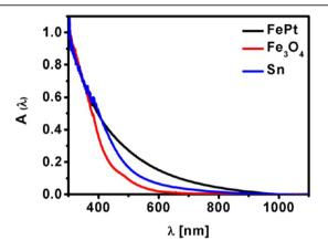
**Figure 88.** Normalized absorption spectra  $A(\lambda)$  of FePt NPs (black curve) (cf. Section 1.4), Fe<sub>3</sub>O<sub>4</sub> NPs (red curve) (cf. Section 1.5), and Sn NPs (blue curve) (cf. Section 1.6). All NPs are dispersed in chloroform. Due to the absence of plasmon resonance, the absorption spectra do not contain defined peaks or characteristics.
