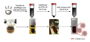
Figure 14. Graphic scheme (upper panel) and photographs (lower panel) of FePt NP purification steps after synthesis.
