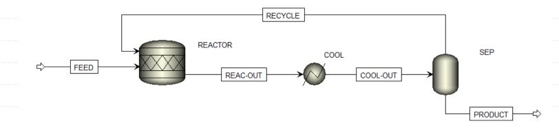
Determine the effect of cooler outlet temperature to achieve a Cumene product purity of 98% mol.
