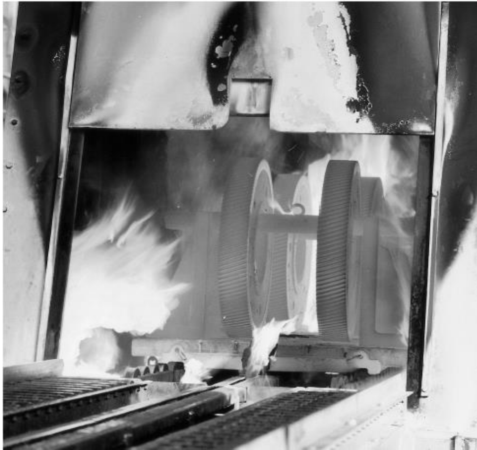
Furnace for heat treating steel using the carburization process. (Courtesy of Cincinnati Steel Treating).
