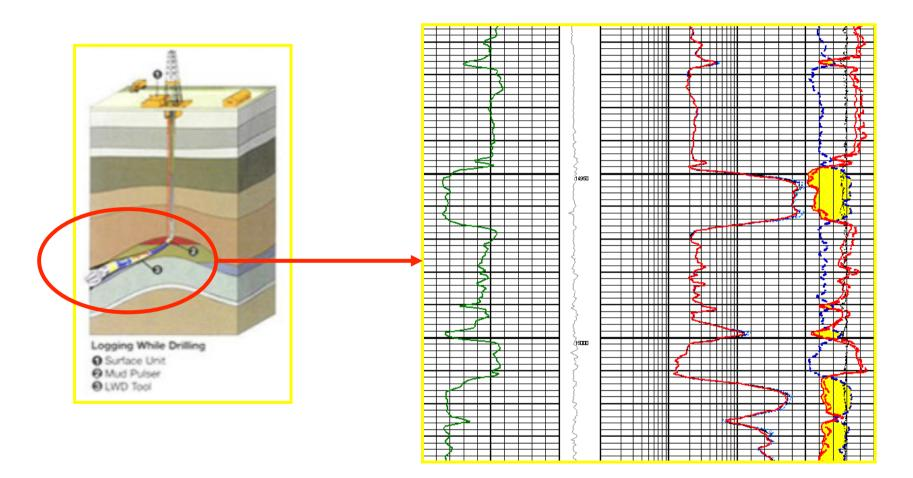
Modern Logging While Drilling technologies allow the acquisition of high quality logging curves (both in Real Time and Memory modes) for Real Time &/or Near Real Time Formation Evaluation and Geosteering.
