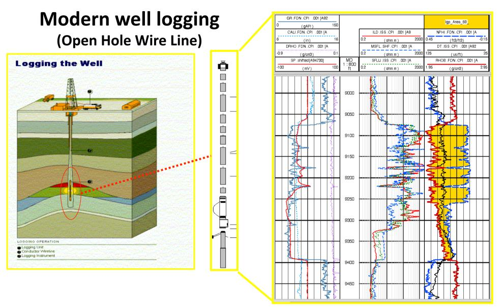
A well log is the product of a survey operation consisting of one or more curves, providing a permanent record of one or more physical measurements as a function of depth in a well bore
