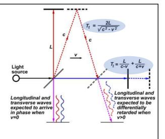
Time difference means **different paths**. An interference will appear. Suppose the apparatus is rotated. Then the fringes will change. **No change!**
