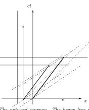
The outward journey. The heavy line is Bob's world line. The dotted line through the origin is the light cone. The dashed lines are the lines of simultaneity in Bob's frame.
