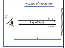
Then when we are at rest with respect to the aether:  $T_0 = \frac{2L_0}{c}$
