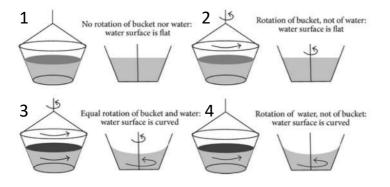
1-3 and 2-4 are examples of same relative motion, yet they are different. The concavity of water is not due to relative motion, but to motion with respect to absolute space.
