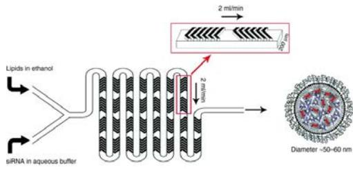
A T-connector apparatus combines fats (dissolved in alcohol) with nucleic acids (dissolved in an acidic buffer)
