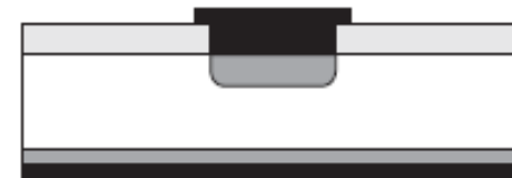
i) ALUMINUM METALLIZATION FOR BACK CONTACT
