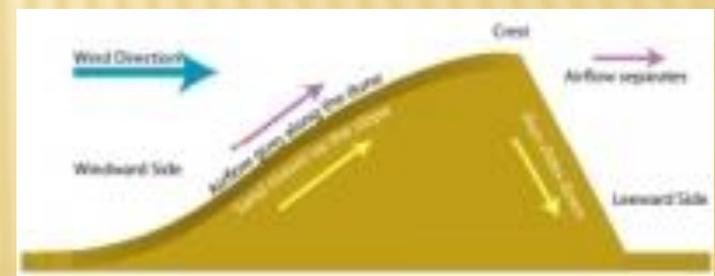
**Figure 2: Illustration of dune cross-section and airflow**
