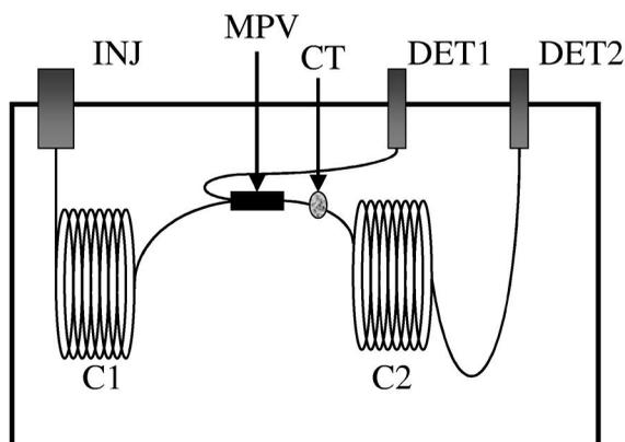
Fig. 7. MDGC instrument schematic. Column 1 (C1) enters the midpoint region and column 2 (C2) is one possible carrier flow exit. When the midpoint valve (MPV) is operated, carrier flows to C2 and heartcut solutes are cryotrapped at CT. The midpoint restrictor connects the midpoint valve to detector 1. INJ: Injector.
