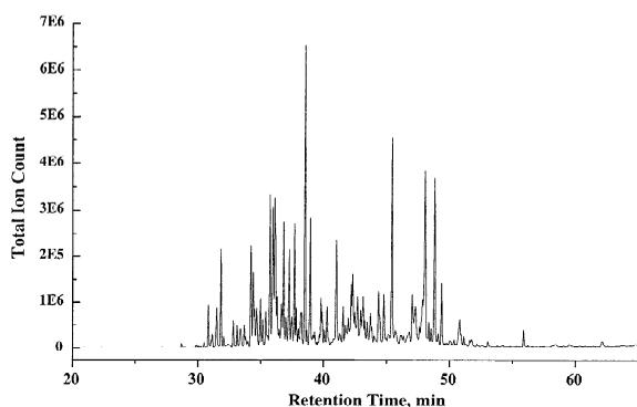
Fig. 10. Typical analysis of *Vetiveria zizanioides* (vetiver) oil by using GC–MS analysis. Agilent 6890GC with a 5730 mass-selective detector, and a BPX5 capillary column (SGE International). Temperature program of 45°C, held for 6 min, then temperature programmed at 3°C/min to 250°C. Initial column head pressure 3.47 p.s.i. (constant flow mode; 1 p.s.i.=6894.76 Pa).
