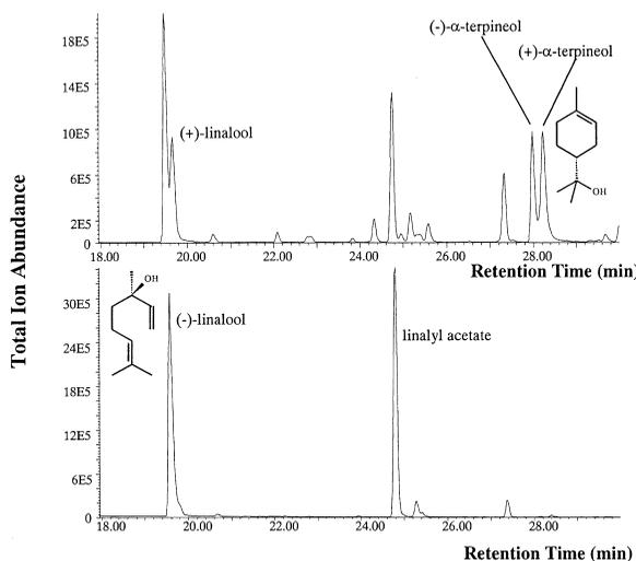
Fig. 4. Chiral chromatograms of Tasmanian lavender oil, showing the simultaneous resolution of ( $\pm$ )-linalool, and ( $\pm$ )- $\alpha$ -terpineol (upper trace). These additional components result from racemisation and rearrangement during acid hydrolysis of the original oil, which is enriched in ( $-$ )-linalool (lower trace). The enantiomeric composition of  $\alpha$ -terpineol was 56% (+)- and 44% ( $-$ )-.
