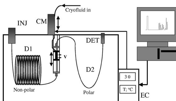
Fig. 9. Schematic diagram of the GC×GC arrangement utilising a cryogenic modulator. CM: Cryomodulator; INJ: injector; DET: detector; D1, D2: separation dimensions 1 and 2; EC: electronic controller with selectable modulation duration (30=3.0 s) and cryotrap temperature shown; V: exit vents from the cryotrap. The modulator oscillates as shown by the arrow. Cryofluid  $\text{CO}_2$  is provided to the trap via the movement arm.
