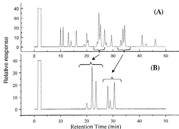
Fig. 6. Multidimensional gas chromatography heartcut concept. Desired regions, which exhibit poor resolution on the first column (A), are transferred to the second column where they are analysed on a more selective phase, which allows their quantitative separation (B).
