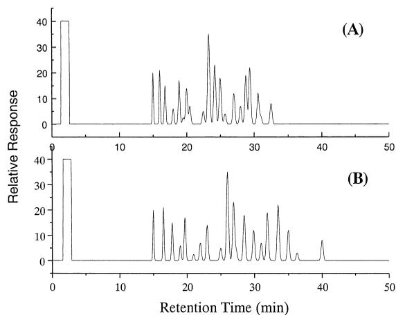
Fig. 2. Illustration of expanded separation space when using a more “selective” column. (A) Compounds are restricted to a small elution (temperature) range for example with a non-polar column. (B) By using a polar (selective) column, compounds with polar groups are retained more strongly and so the total sample will be spread over a greater elution range. This leads to better apparent resolution.
