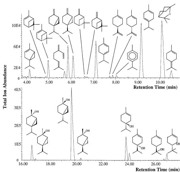
Fig. 3. The monoterpene hydrocarbon and oxygenated monoterpene region (upper and lower traces, respectively) of a chromatogram (determined on a commercial chiral column, J&W CyclodexB, 30 m×0.25 mm I.D., 0.25  $\mu$ m film thickness) from a typical sample of flush growth from *Melaleuca alternifolia*.
