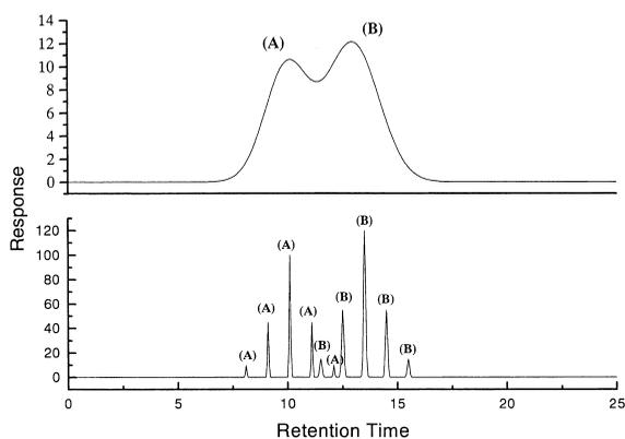
Fig. 12. Conceptual representation of resolution of two peaks which are unresolved on the first column (top) but by the pulsing process and orthogonal analysis conditions are resolved on the second column (bottom). When using a mass spectrometer, peaks labelled (A) will all be identified by library searching as the one component, and those labelled (B) will be the other component.
