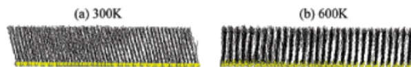
Figure 3. Snapshots of alkanethiol [\text{SH}-(\text{CH}_2)_{13}-\text{CH}_3] SAMs from our MD simulations at (a) 300 and (b) 600 K.
