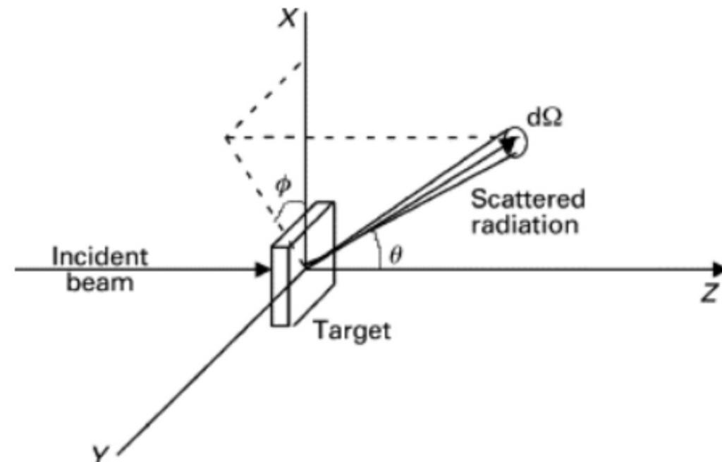
$$\sigma = \int \frac{d\sigma}{d\Omega} d\Omega = \int_0^\pi \sin\vartheta d\vartheta \int_0^{2\pi} \frac{d\sigma}{d\Omega} d\varphi$$
