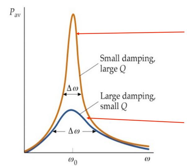
When damping is small oscillator absorbs much more energy from driving force.
