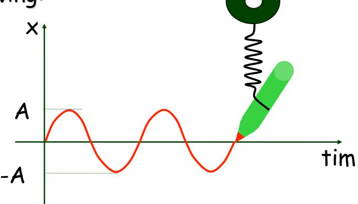
The general equation for the curve traced out by the pen is  $x = A \cos(\omega t + \delta)$
