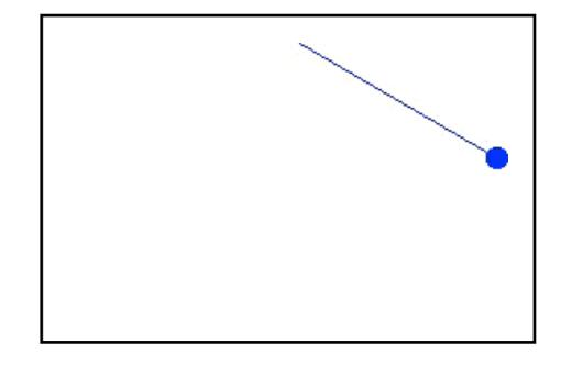
$$T = T_{o} \left(1 + \left(\frac{1}{2}\right)^{2} \sin^{2}\left(\frac{\phi}{2}\right) + \left(\frac{1}{2}\right)^{2} \left(\frac{3}{4}\right)^{2} \sin^{4}\left(\frac{\phi}{2}\right) + ....\frac{1}{7}\right)^{2}$$
