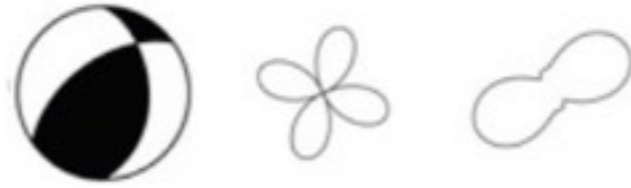
Focal mechanism and radiation pattern
