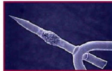
Single oriented W crystal fine tip
