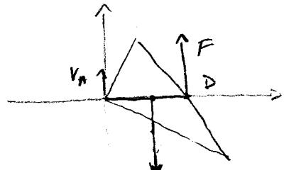
$$\text{se } \lambda < 1 \quad \varphi^{(1)} = -\varphi^{(2)}, \text{ stabile}, \begin{cases} H_A = -F \sqrt{1-\lambda^2} < 0 \\ V_A = mg - F \lambda \end{cases}$$
