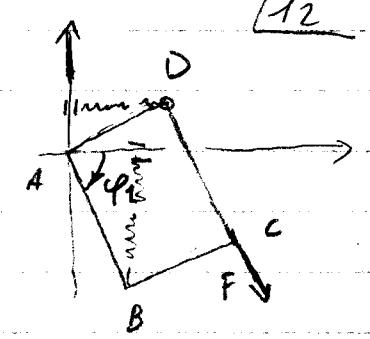
$$\varphi_2 = \varphi, \quad \left\{ \begin{array}{l} H_A = 4cl \sqrt{\frac{1-\sqrt{1-\lambda^2}}{2}} - F \sqrt{\frac{1+\sqrt{1-\lambda^2}}{2}} \\ V_A = (3cl - F) \left( -\sqrt{\frac{1-\sqrt{1-\lambda^2}}{2}} \right) \end{array} \right.$$
