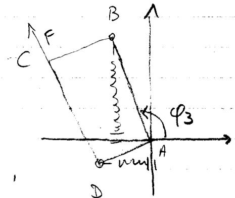
$$\varphi_4 = \pi + \varphi, \quad \left\{ \begin{array}{l} H_A = -4cl \sqrt{\frac{1-\sqrt{1-\lambda^2}}{2}} + F \sqrt{\frac{1+\sqrt{1-\lambda^2}}{2}} \\ V_A = (3cl - F) \sqrt{\frac{1-\sqrt{1-\lambda^2}}{2}} \end{array} \right.$$
