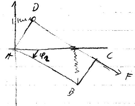
$$\varphi_3 = \frac{\pi}{2} - \varphi, \quad \left\{ \begin{array}{l} H_A = -4cl \sqrt{\frac{1+\sqrt{1-\lambda^2}}{2}} + F \sqrt{\frac{1-\sqrt{1-\lambda^2}}{2}} \\ V_A = (3cl - F) \sqrt{\frac{1+\sqrt{1-\lambda^2}}{2}} \end{array} \right.$$
