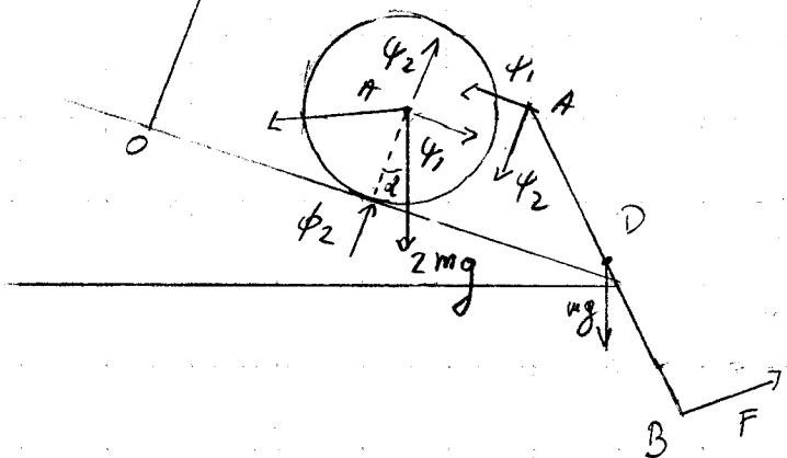
$$\begin{aligned} \vec{R} \cdot \vec{e}_1 &: \quad \left\{ \begin{array}{l} -C \phi_2 + 2mg \sin \alpha + \psi_1 = 0 \\ -C R - 2mg \cos \alpha + \psi_2 + \phi_2 = 0 \end{array} \right. \\ \vec{R} \cdot \vec{e}_2 &: \end{aligned}$$
