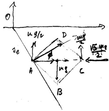
$$\vec{q}_e^{(2)} = \left( \frac{mg}{\sqrt{3}c}, 0 \right), \vec{\phi} = \frac{mg}{2} (\sqrt{3} \vec{e}_x + \vec{e}_y)$$
