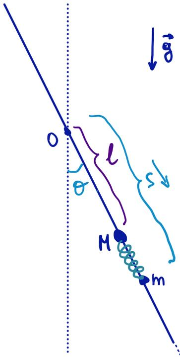
$$\begin{aligned}x_o &= l \sin \theta & \dot{x}_o &= l \dot{\theta} \cos \theta \\y_o &= -l \cos \theta & \dot{y}_o &= l \dot{\theta} \sin \theta\end{aligned}$$
