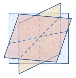
Considering the projection theorem, each FT of a projection includes the center of the Fourier space.
