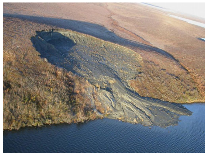
Fig. 24 A flowslide caused by multiple retrogressive failure of ice-rich permafrost (a thaw flow) in the Mackenzie Region, North-west Territories, Canada (Courtesy of B. Wang, Geological Survey of Canada)
