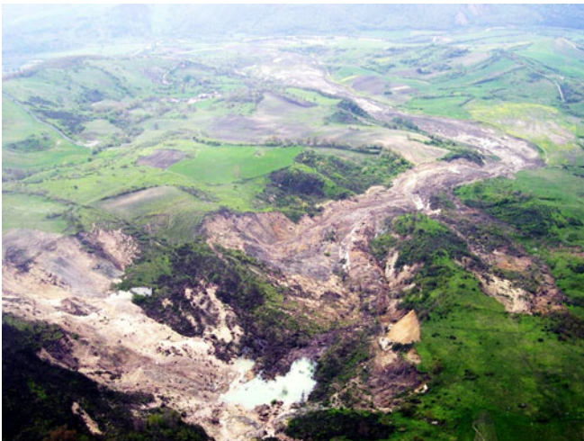
Fig. 34 An earthflow surge initiated by a planar slide in the Campania Region, Italy (Courtesy of F. Guadagno University of Sannio, Benevento)
