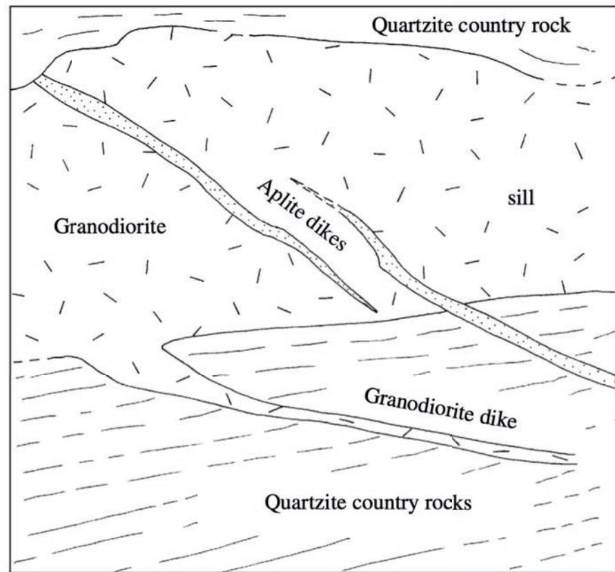
9.3 Sill and dikes. A **sill** of granodiorite intruded concordantly with layering in quartzite host rock and a smaller offshoot **dike** penetrating discordantly across layering. Thin subparallel dikes of leucocratic granite aplite cut across more mafic granodiorite and layered country rock. Note sharp contacts. Camera lens cap in lower left for scale. (a) Photograph. (b) Annotated sketch.
