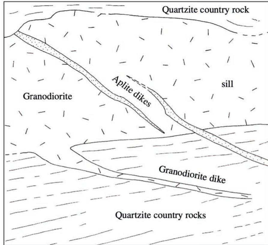
9.3 Sill and dikes. A **sill** of granodiorite intruded concordantly with layering in quartzite host rock and a smaller offshoot **dike** penetrating discordantly across layering. Thin subparallel dikes of leucocratic granite aplite cut across more mafic granodiorite and layered country rock. Note sharp contacts. Camera lens cap in lower left for scale. (a) Photograph. (b) Annotated sketch.
