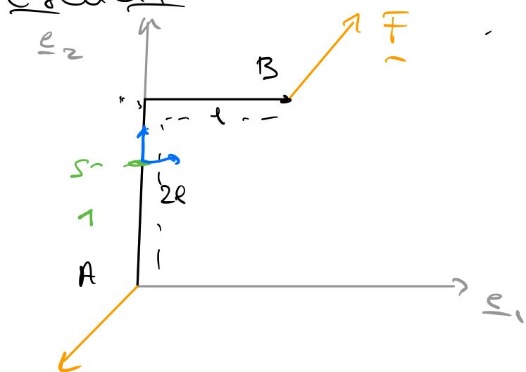
$$\underline{F} = \underline{F}_{\text{ver}} (\underline{x}_B - \underline{x}_A)$$
