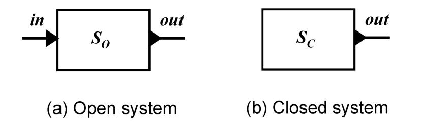
For verification, we obtain a closed system by composing the system and environment models
