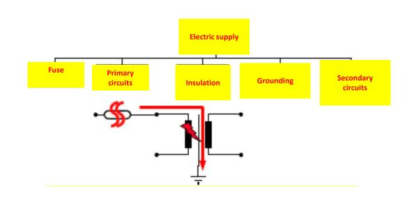
Faults in the "insulation" cause "overload" which consequentely causes the fuse to "open".
