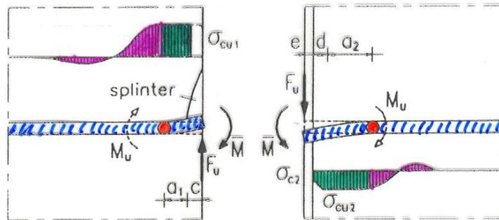
$$\left\{ \begin{array}{l} F_u = \sigma_{cu1} \cdot \phi \cdot a_1 \\ M_u = F_u \cdot (a_1 + c) - \frac{\sigma_{cu1} \cdot \phi \cdot a_1^2}{2} - \bar{M} \\ F_u = \sigma_{cu2} \cdot \phi \cdot (a_2 + d) - (\sigma_{cu2} - \sigma_{c2}) \cdot \phi \cdot \frac{d}{2} \\ M_u = F_u \cdot (a_2 + d + e) - \sigma_{cu2} \cdot \phi \cdot \frac{(a_2 + d)^2}{2} + \\ \quad + (\sigma_{cu2} - \sigma_{c2}) \cdot \phi \cdot \frac{d}{2} \left( a_2 + \frac{2d}{3} \right) + \bar{M} \end{array} \right.$$
