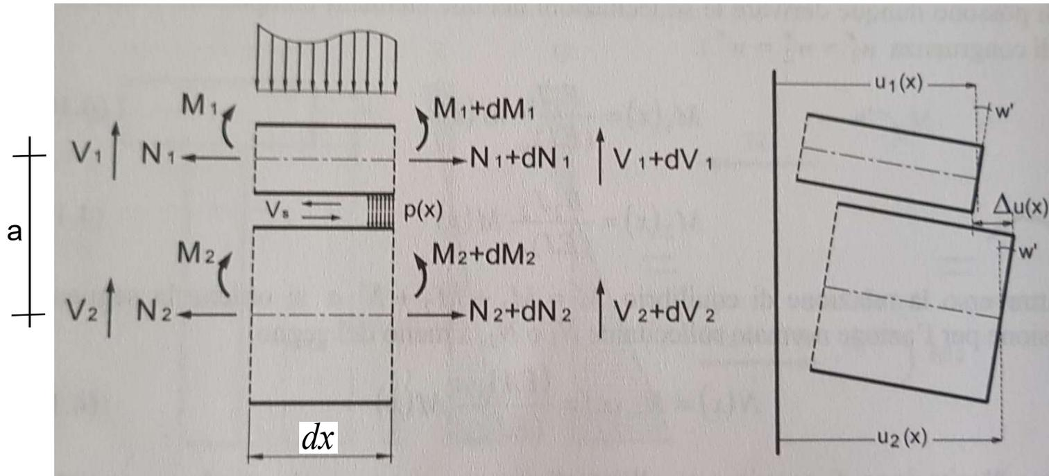
$$\frac{dN_c}{dx} = E_c A_c u''_c \quad \frac{dN_s}{dx} = E_s A_s u''_s \quad \frac{dV_c}{dx} + \frac{dV_s}{dx} = p$$
