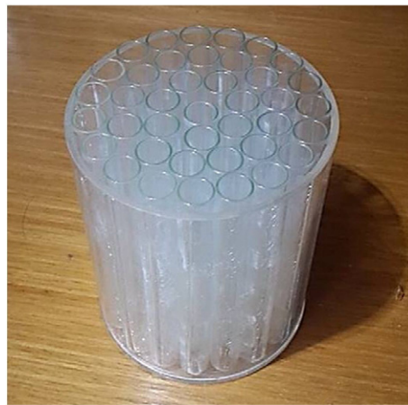
Fig. 12. By dividing the cup into smaller cylindrical cells, we can displace the oscillation from resonance.
