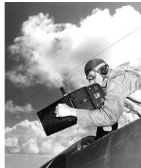
After 1917 the Fairchild's camera was invented by Sherman M. Fairchild. His camera major improvement was a shutter located inside the lens, able to significantly reduce image distortion caused by slow shutter speeds and becoming the standard camera system for many decades.
