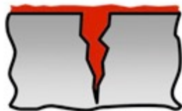
3 Application of penetrant
