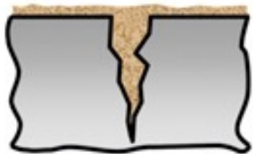
1 Crack filled with dirt
