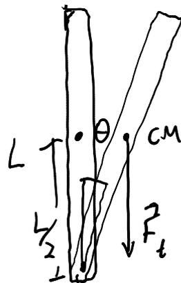
$$\begin{aligned}\tau &= \vec{r} \times \vec{F} \\ &= r F_t \sin \theta \\ &= \frac{L}{2} mg \sin \theta\end{aligned}$$
