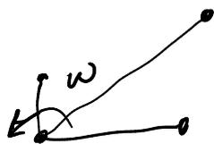
$$K = \sum_i \frac{1}{2} m_i v_i^2 = \sum_i \frac{1}{2} m_i (\omega r_i)^2 = \frac{1}{2} \underbrace{\sum_i m_i r_i^2}_{I} \omega^2$$
