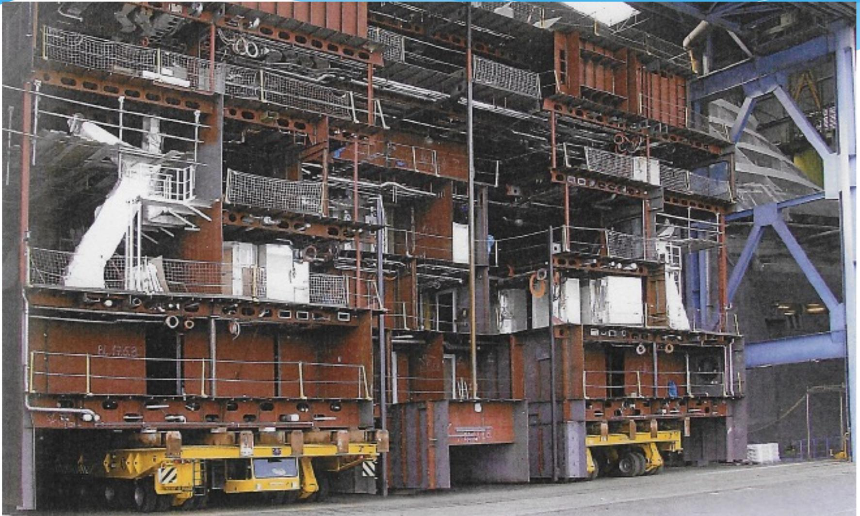
*The blocks and sections are already equipped with cable systems, pipes, A/C shafts etc. to make great productivity progress.*
