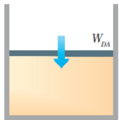
$$W_{DA} = -\Delta U_{DA} = m c_v (T_1 - T_2) = -W_{BC}$$
