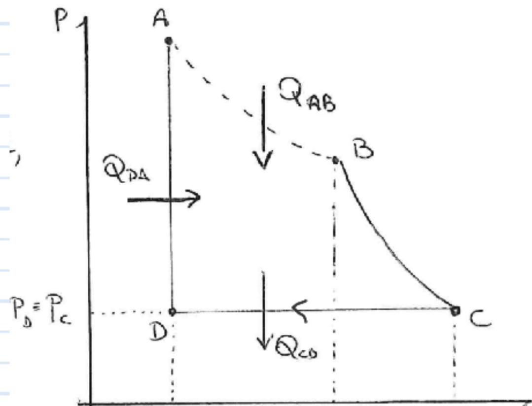
$$W_{BC} = -\Delta U_{BC} = -m C_V (T_C - T_B) = m C_V (T_B - T_C)$$
