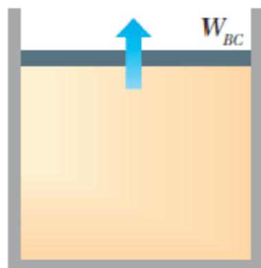
$$W_{BC} = -\Delta U_{BC} = m c_v (T_2 - T_1)$$
