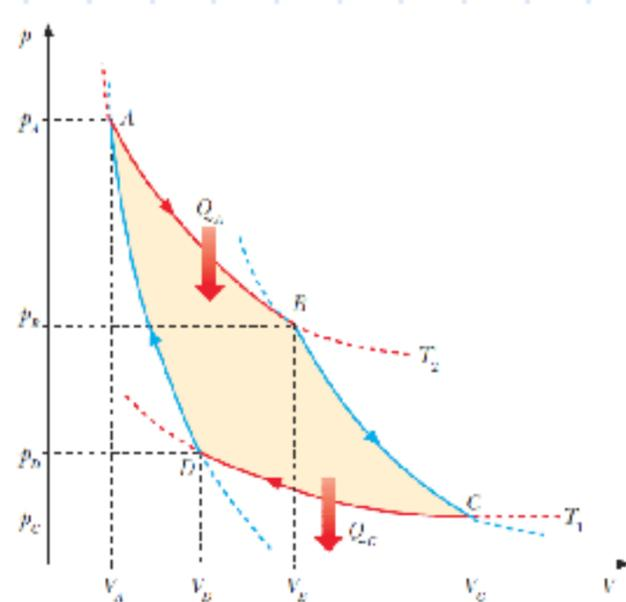
$$\overline{DA} : Q = 0 \quad T_2 V_A = T_1 V_D$$
