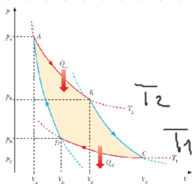
$$\overline{BC} : Q = 0 \quad T_2 V_B^{\gamma-1} = T_1 V_C^{\gamma-1}$$
