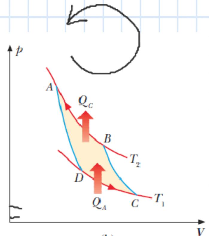
$$\frac{V_B}{V_A} = \frac{V_C}{V_D} = \frac{T_1}{T_2 - T_1}$$
