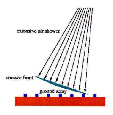
Reconstruction of the γ direction with the particles arrival times
