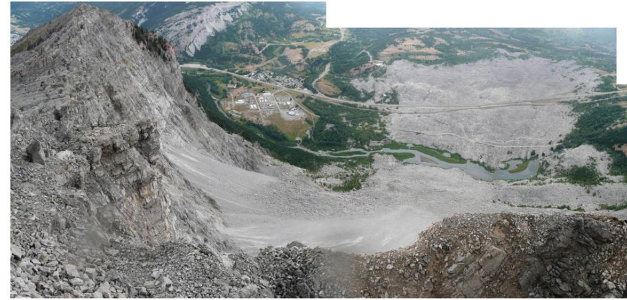
Fig. 19 "Frank Slide" rock avalanche of 1903, southern Alberta, Canada. The horizontal length of the avalanche path is 3 km, volume 36 million m 3 . (Photo by O. Hungr)
