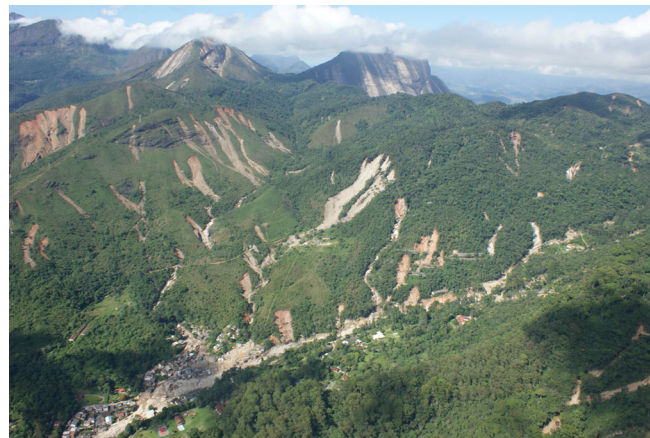
Fig. 33 A cluster of debris avalanches and debris flows of January, 2010 in the Serrana Region of Brazil (Courtesy of A.L. Coelho-Netto, Federal University of Rio de Janeiro)
