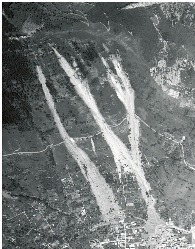
Fig. 32 Several of the catastrophic debris avalanches of May, 1998 in Siano, Italy, illustrating the characteristic widening of debris avalanche scars on steep slopes (Vertical airphoto published by licence no. 2347-02/December/2002 of Regione Campania. Image courtesy of Dr. P. Revellino, University of Sannio, Benevento)
