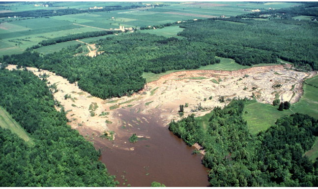
Fig. 25 A flowslide in sensitive clay, Lemieux, Ontario, Canada (Courtesy of S.G. Evans, University of Waterloo)
