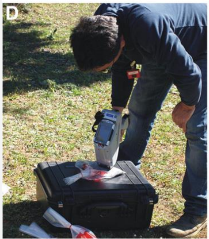
XRF set up for field analysis
