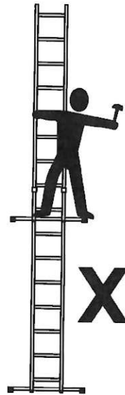
Figure 32 — Example of a hazard in use with a two section extension ladder where the sections may be separated
