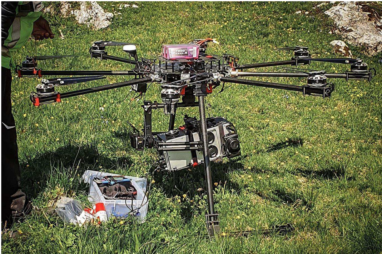
Figure 4. Image of the UAV and HySpex Mjolnir-VS mounted sideways in the Gremsy gStabi H16 XL gimbal. Lens caps for the three sensors (VS-1240, S-620 and Sony Alpha) can be seen on the right side of the camera.
