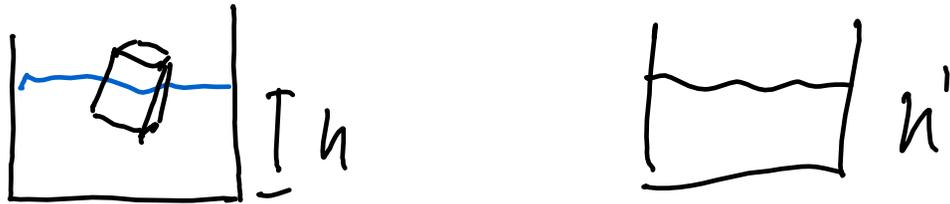
$$\rho_g V_{\text{Tot}} = \rho V_{\text{imm}} \quad \downarrow \quad V_{\text{imm}} = \frac{\rho_g}{\rho} V_{\text{Tot}}$$
