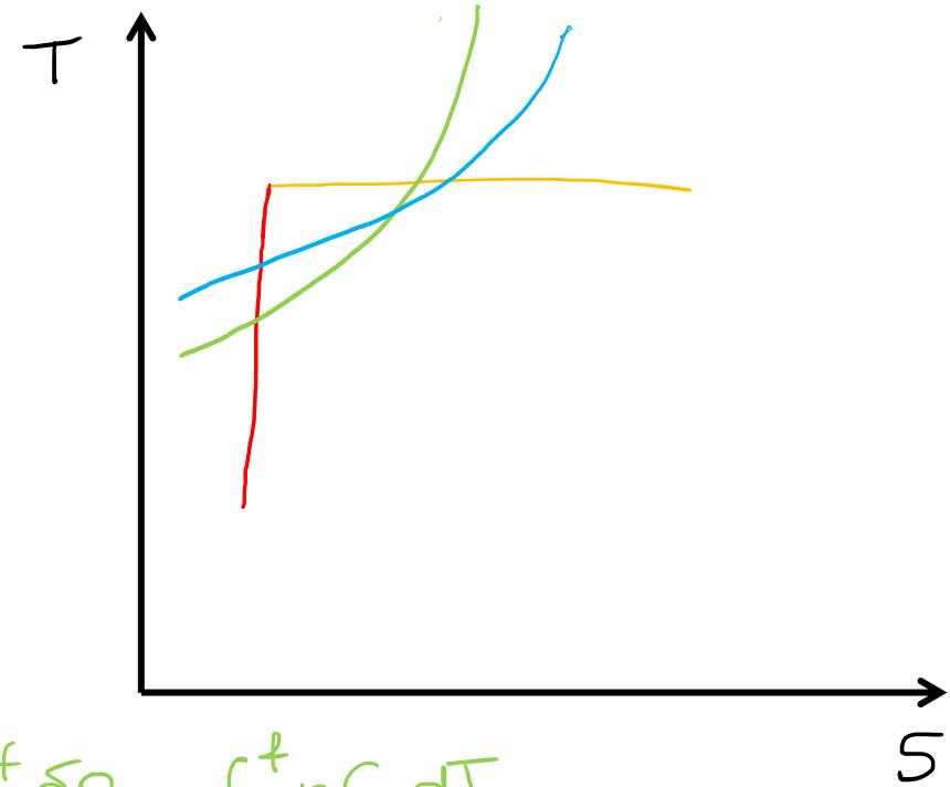
$$\int_{i, \text{rev}}^f \frac{\delta Q}{T} = \int_{i, \text{rev}}^f \frac{n C_v dT}{T} =$$
